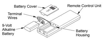
Figure 39 - Installing Alkaline Battery in Hand-Held Remote Control Unit (GHRCB)
